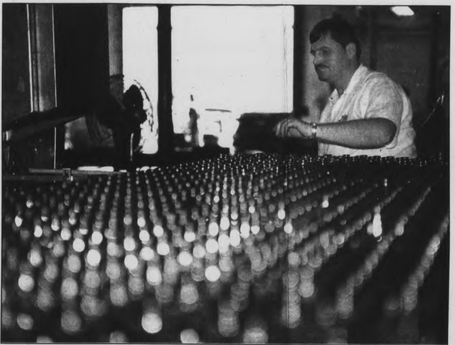
An Ale-8-One employee watches empty bottles move on to the conveyor belt. On a typical day, he might see as many as 400 bottles a minute.
