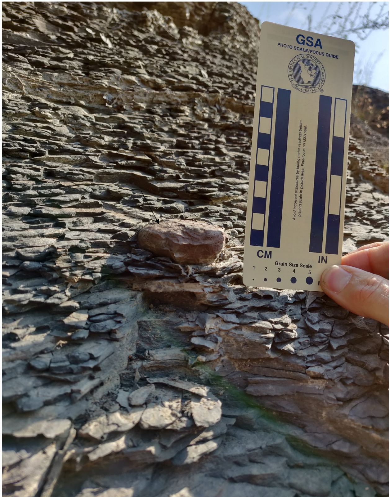
FI-A: Siderite nodules observed at 7.92 m in lithologic unit 2 within Upward-coarsening Sequence 1.
