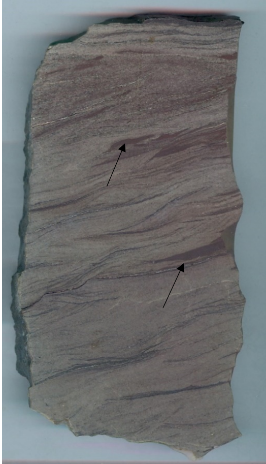
CI-B: Medium gray sandstone collected from 18.94 m within Coarsening-upward Sequence 1 (lithologic unit 8). Note thick to thin internal cross lamination and prominent mud drapes up to 3 mm thick.
