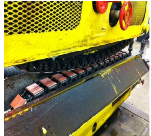
FIGURE 3: LEGACY MACHINE, “CHAIN STYLE TRACTOR” – MUST BE ADJUSTED MANUALLY
