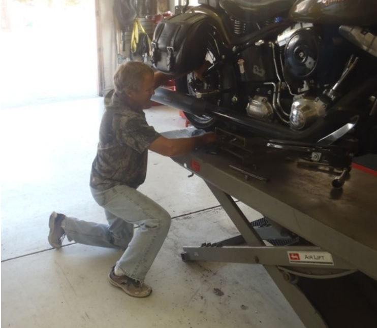
Figure 5, Kneeling Posture: The low height of the motorcycle rack forces the repair professional to kneel to perform the necessary work.
