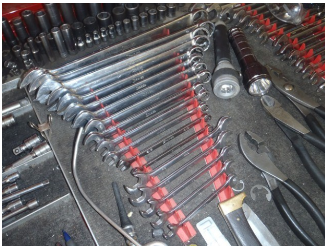
Figure 4, Tools: Standard box end wrenches used on a daily bases where force is applied on the narrow part of the wrench, placing soft tissue compression onto the palm and or fingers of the hand.
