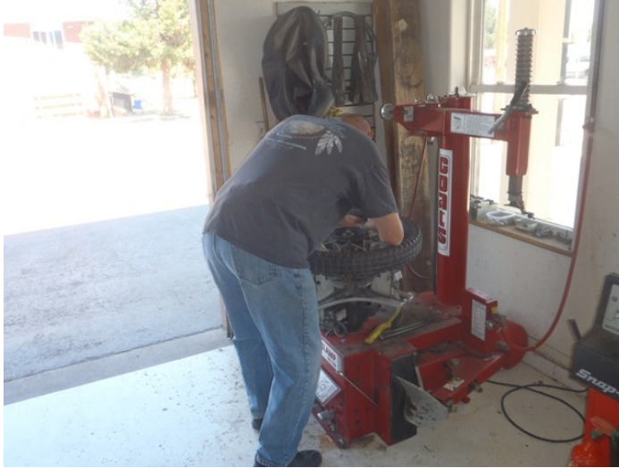
Figure 3, Tire Machine Posture: A repair professional is replacing a tube on a metric motorcycle wheel and tire assembly.
