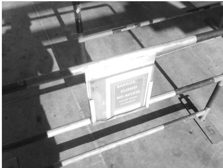
Figure 4. Typical Barrier for Lifting Operations. This is a typical barrier is used to close access to areas on the rig. Barriers restrict access due to overhead operations.
