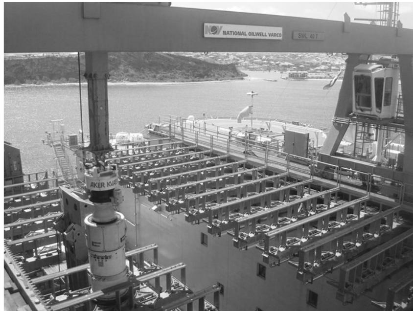
Figure 3. Rig's Riser Bay. Risers connect the rig to the ocean floor via the BOP and well head.
