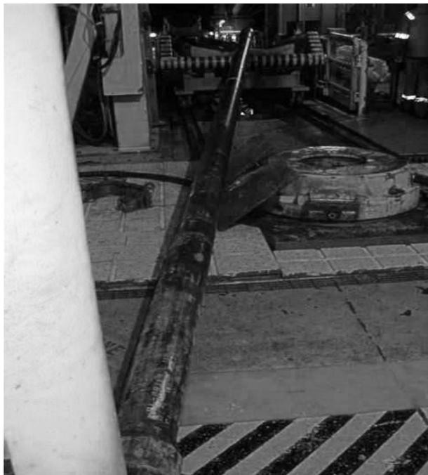
Figure 7. Dropped Casing. The dropped casing is seen in the picture lying across the red zone.
