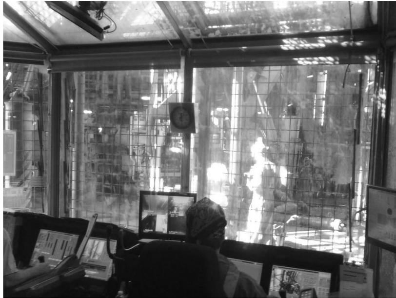
Figure 5. Cyber Chair. View from inside the dog house to the drill floor. Drillers are sitting in Cyber Chairs.
