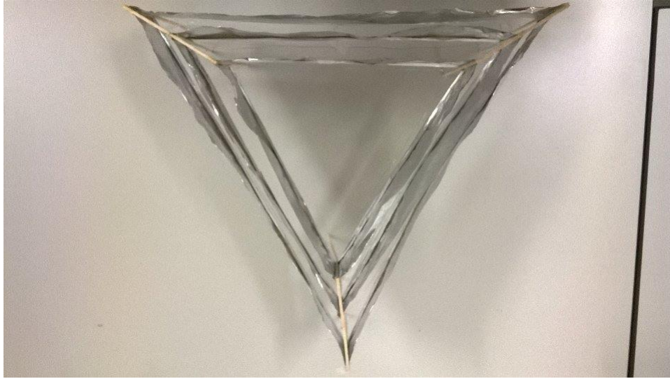
Figure IX - Triple Triangular Craft: Weight increased and more arcing present. The arcing was specially observed in between the cathodes.
