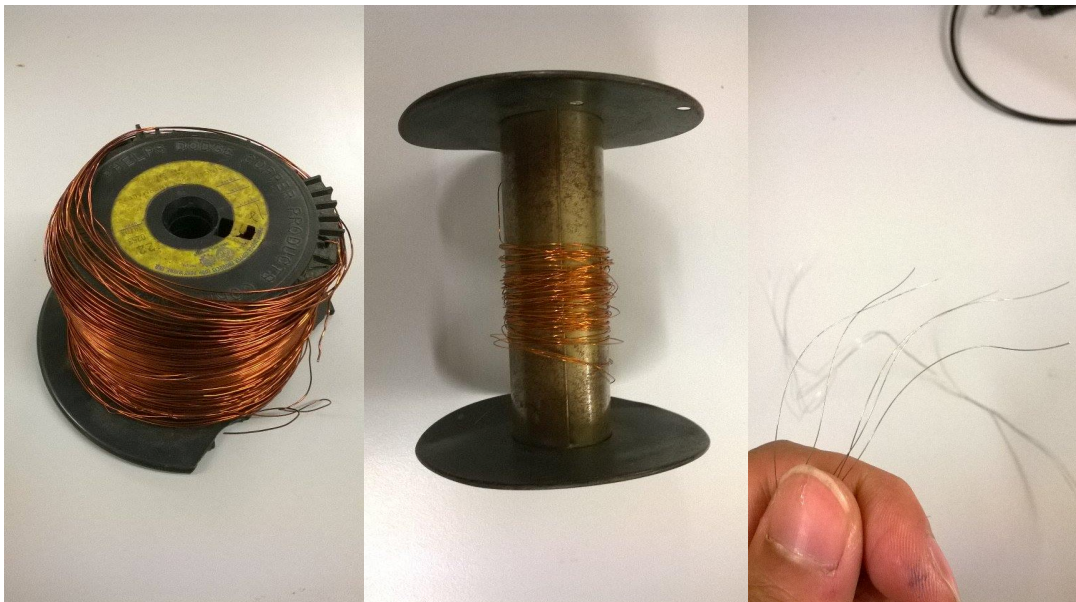
Figure IV - The copper wire in this craft was too thick. After the changes, the Copper Wire was insulated; this insulation prevented the ionization of air. It was later found that the stainless steel wire worked the best due to its tensile strength when dealing with thin wires.
