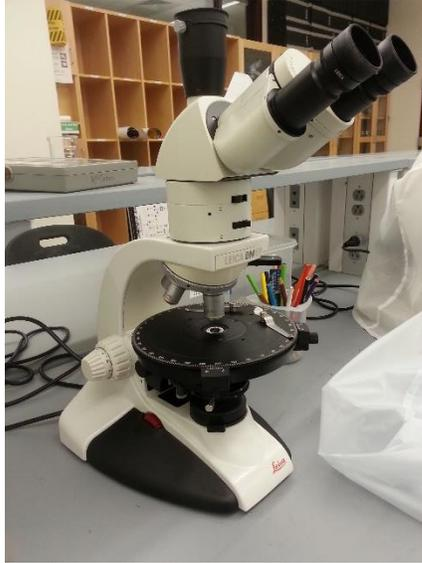
**Figure 5.1.** Leica DM EP Polarized Light Microscoped used to visually observe lignin-IL interactions.
