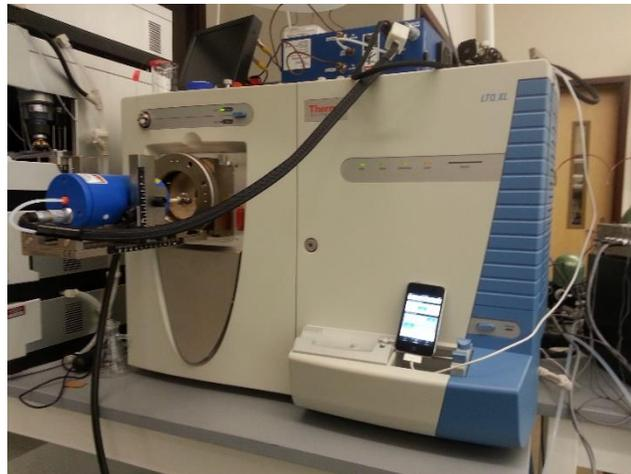
**Figure 5.2.** Thermo Scientific LTQ XL with DART ion source used to characterize lignin-IL interactions.
