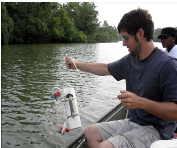
Figure 5. Van Dorn sampler (left) and grab sampler (right).
