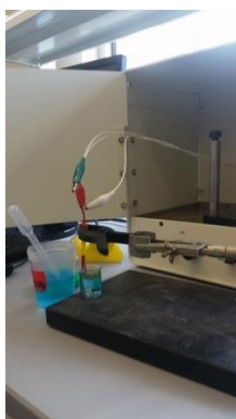
Figure 3.2: Image of the potentiostat and metal solution setup
