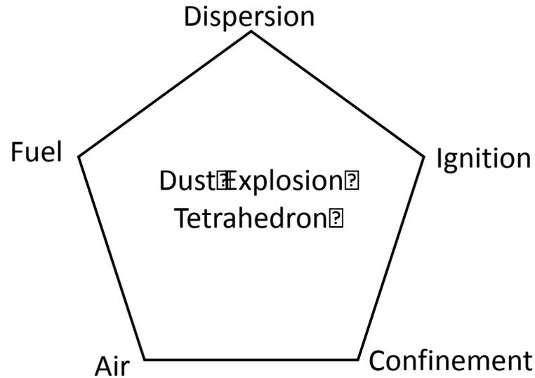
Figure 2: Dust Explosion Tetrahedron
