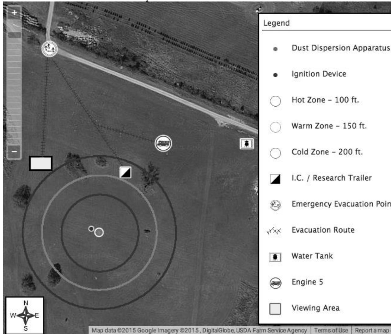
**NOTE:** HOT, WARM, & COLD Zone distances determined by Hydrocarbon Fireball Calculations in APPENDIX 4.
