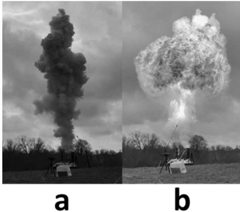
Figure 5: Test using 4.55kg of Woodmeal.
