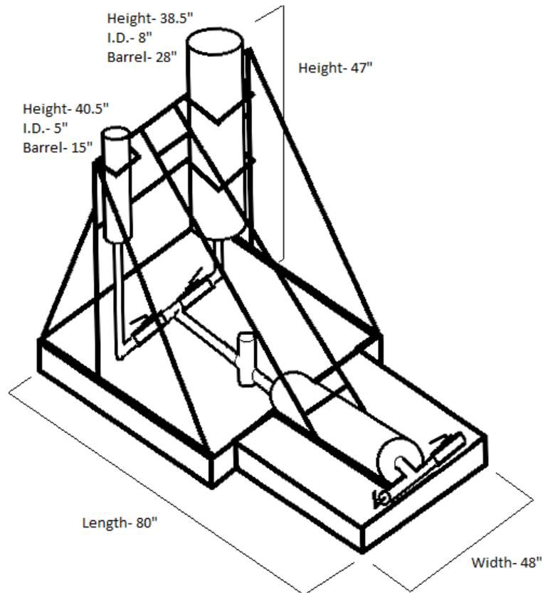
Figure 3: Dust Dispersion Apparatus Design
