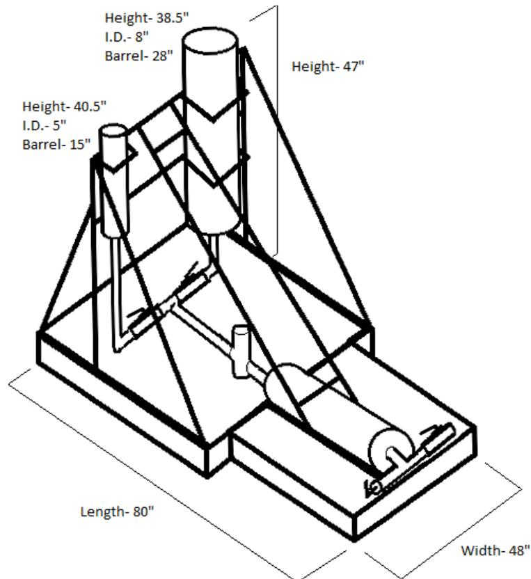
Figure 3: Dust Dispersion Apparatus Design
