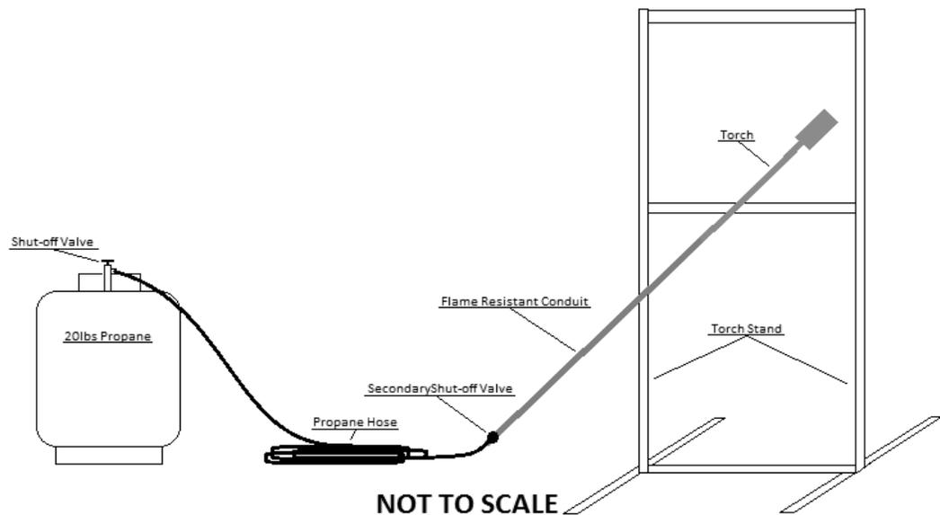
Figure 4: Propane Ignition Device
