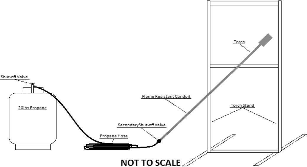
Figure 4: Propane Ignition Device
