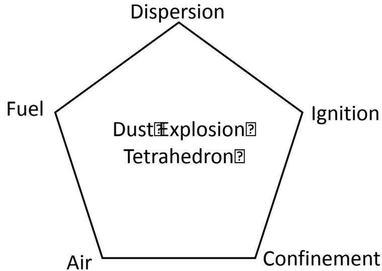
Figure 2: Dust Explosion Tetrahedron
