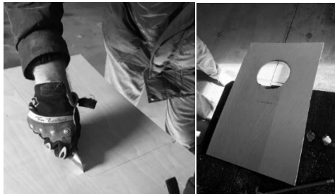
Figures 13: Cutting out the Top of the Sound Box and the Sound Hole
