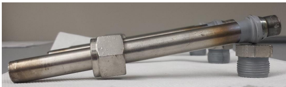
Figure 2-1. Steel vessel used for housing the aqueous amine solutions loaded with CO 2 for thermal degradation.
