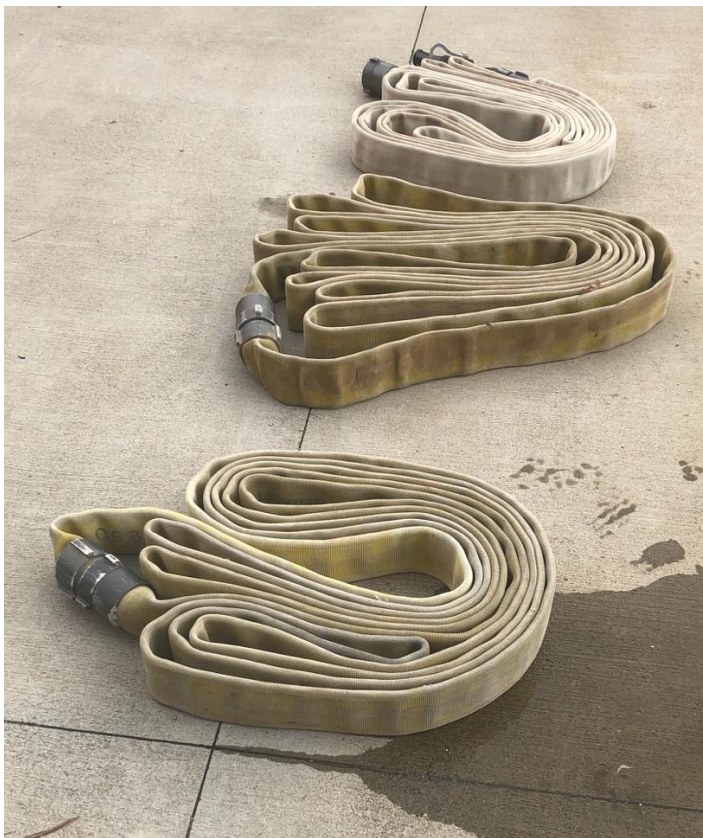
Three fifty-foot long sections of hose in the Denver Load prepared for the next replicate.
