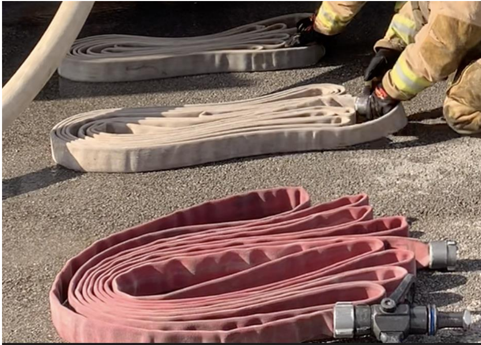
One-and-three-quarter-inch hose bundles before being deployed.
