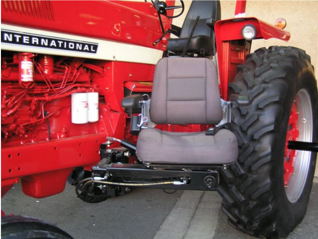
Image 3 Chair lift on an International tractor (University of Kentucky College of Agriculture, 2019)
