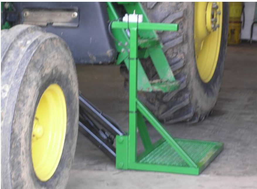
Image 2 Standing lift on a John Deere tractor (University of Kentucky College of Agriculture, 2019)
