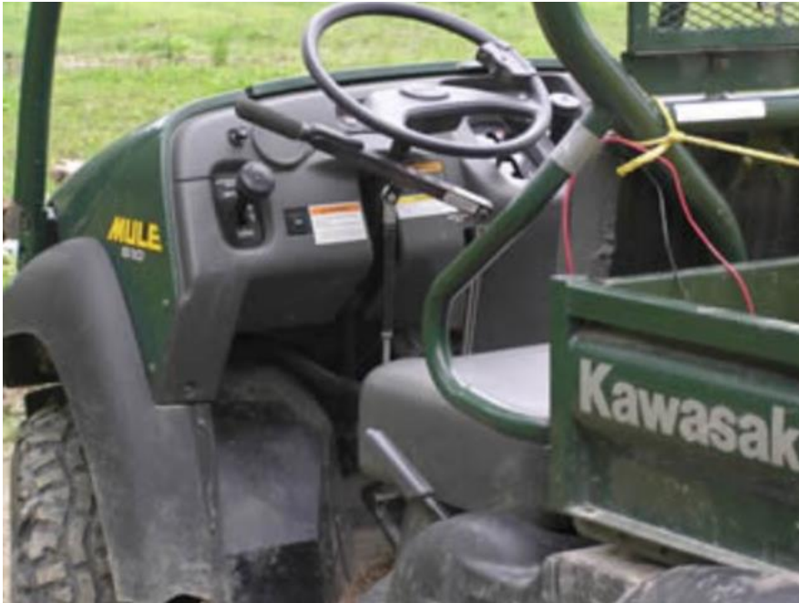
Image 1 Hand controls on a Kawasaki Mule (University of Kentucky College of Agriculture, 2019)
