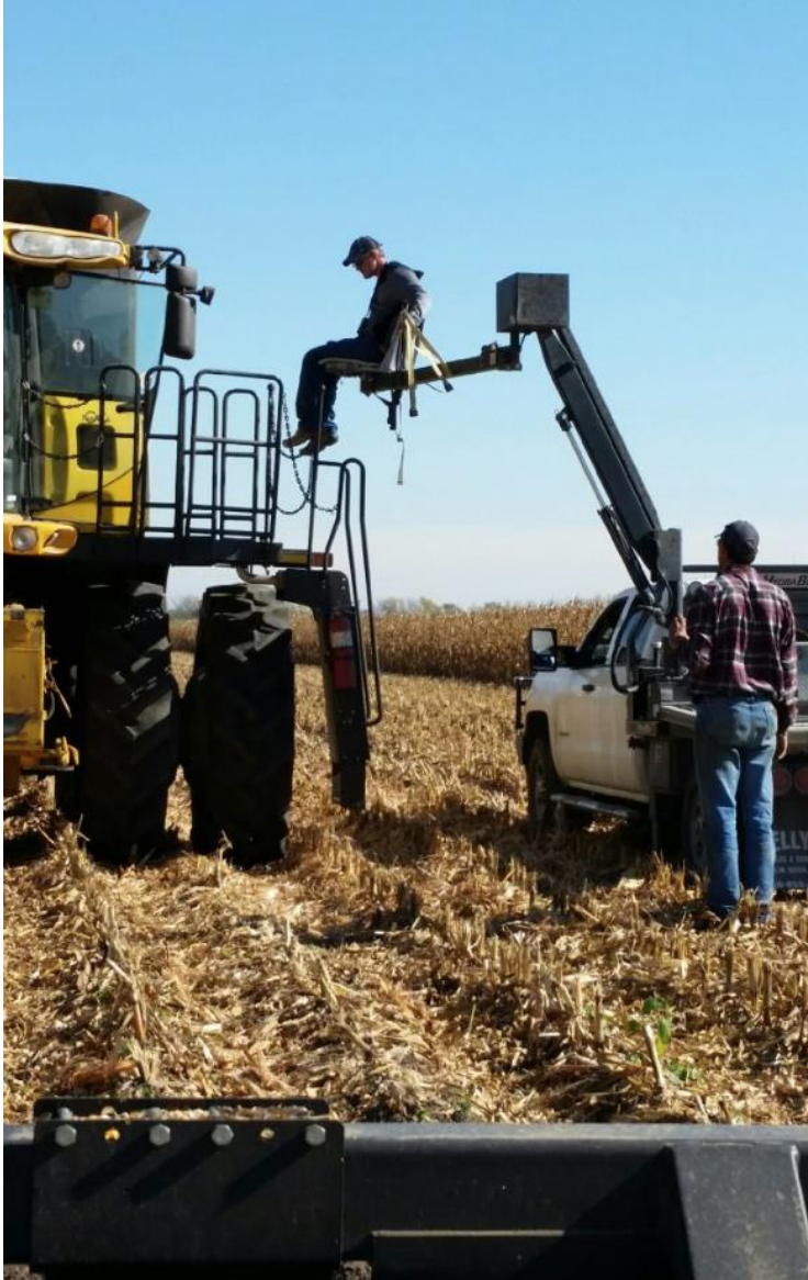
Image 4 Chair lift on pickup truck being used to allow farmer to enter combine without ladder use (Lensegrav & Choat, 2018).
