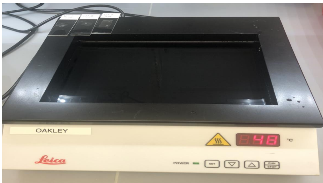
Figure 6. Leica HI1210 water bath with a surface that provides high thermal conductivity rates.
