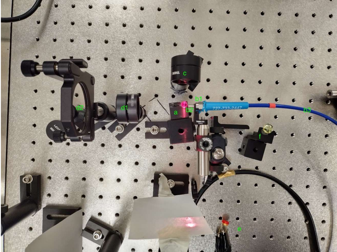
Figure 5: Initial Setup of Alexandrite Excitation Experiment with (a) Alexandrite Crystal, with Visible Fluorescence from a Columnar Region, (bX) Elements of Optical Fiber Connected to USB Spectrometer, (b1) Metal Ferrule of Optical Fiber, (b2) Optical Fiber Tip, (b3) Soft Plastic Jacket for Optical Fiber, (c) Focusing Lens; (dX) Additional Optical Elements, (d1) Collimating Lens and (d2) Retroreflector 2" Mirror, (e) Photodiode, Out of its Mount, (f) Uranium Glass Bead
