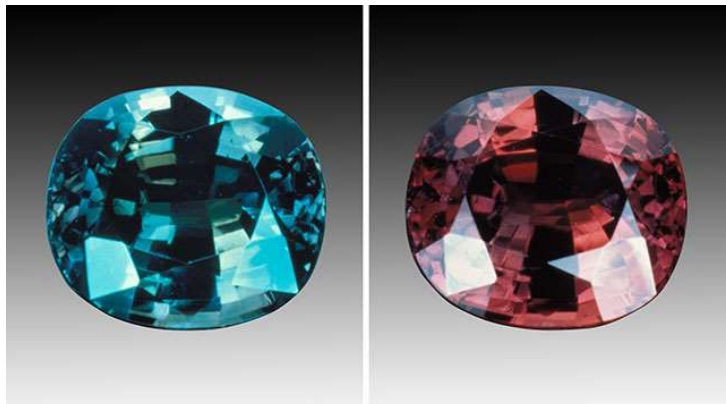
Figure 1: Russian Alexandrite Sample Color Change under Daylight (Left) and Fluorescent Light (Right)
