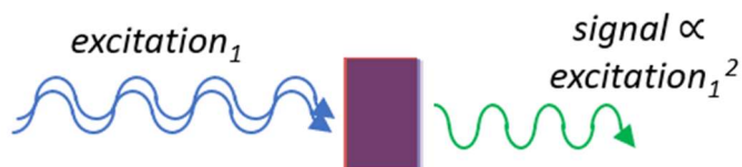
Illustration 3: Illustration of Wavelengths from the Same Source Passing Through a Sample and Creating a Signal Proportional to the Wavelength Squared
