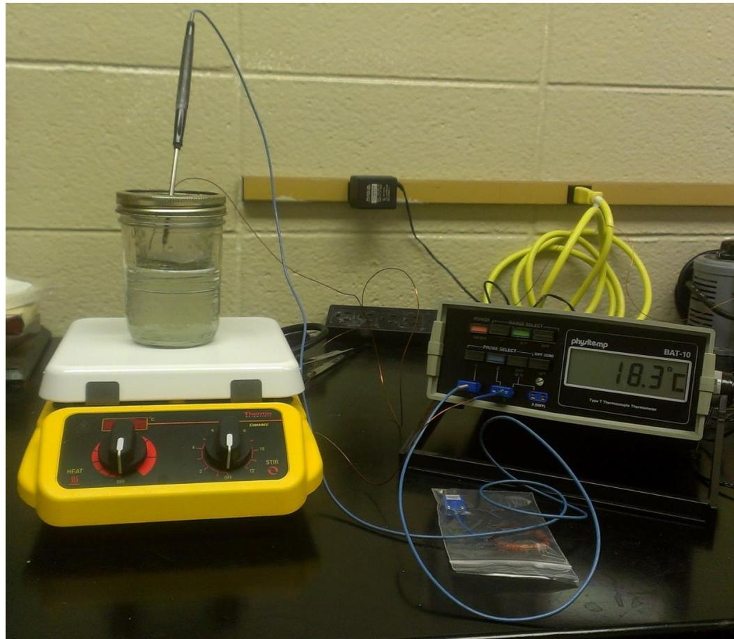
Figure 2: Critical Thermal Maxima Testing Apparatus
